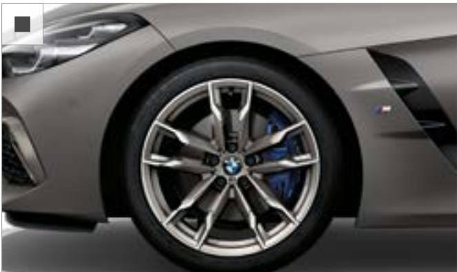
19" M light alloy Double-spoke style 800 M wheels, Bicolour Cerium Grey, front 9 J x 19 with 255/35 ZR19, rear 10 J x 19, 275/35 ZR19 tyres. Standard on M40i models.
