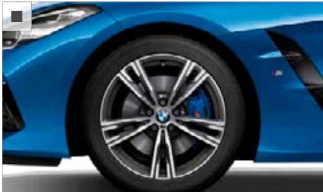
18" M light alloy Double-spoke style 798 M wheels, Bicolour Ferric Grey, front 8 J x 18 with 225/45 ZR18, rear 9 J x 18, 255/40 ZR18 tyres. Standard on M Sport models.
