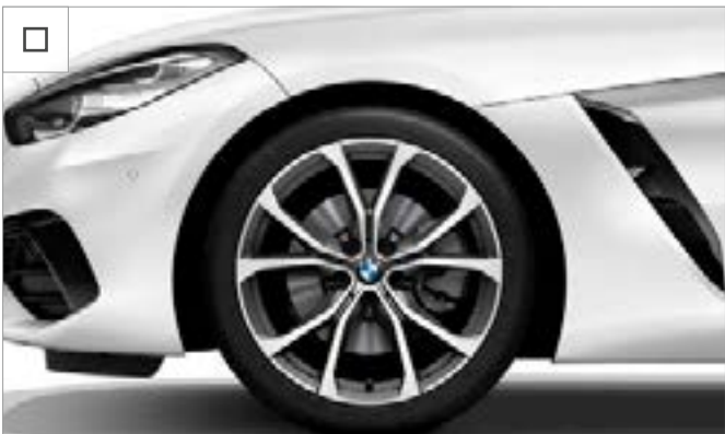
19" light alloy V-spoke style 772 wheels, Bicolour Ferric Grey, front 9 J x 19 with 255/35 ZR19, rear 10 J x 19 with 275/35 ZR19 tyres. Optional on Sport models.
