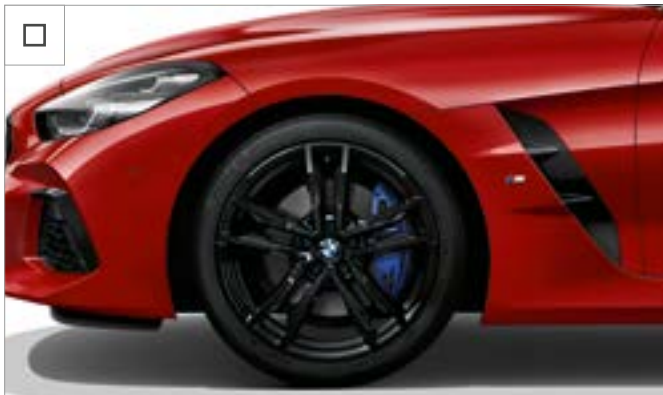
19" M light alloy Double-spoke style 799 M wheels, Jet Black, front 9 J x 19 with 255/35 ZR19, rear 10 J x 19 with 275/35 ZR19 tyres. Only available with Shadowline Plus.
