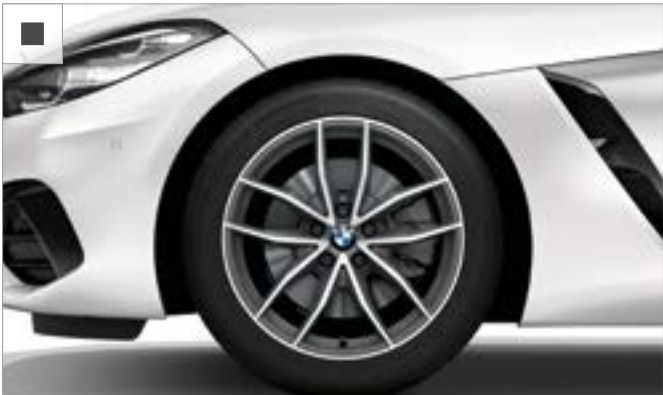
18" light alloy V-spoke style 770 wheels, Bicolour Orbit Grey, front 8 J x 18 with 225/45 ZR18, rear 9 J x 18 with 255/40 ZR18 tyres. Standard on Sport models.
